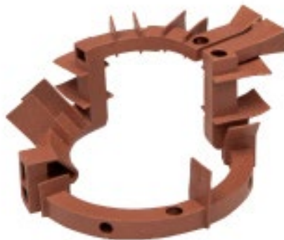
3D CAD model and final 3DPCoil for wheel hubs without brazed joints
