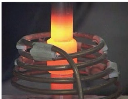
Brazing in a protective atmosphere
