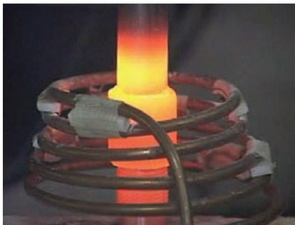
Brazing in a protective atmosphere
