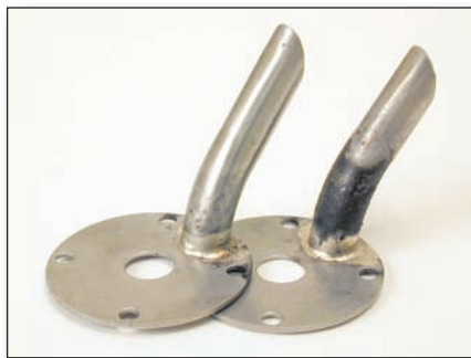
A controlled atmosphere eliminates oxidation.
