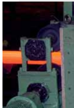
8.000 KW normalizing line
